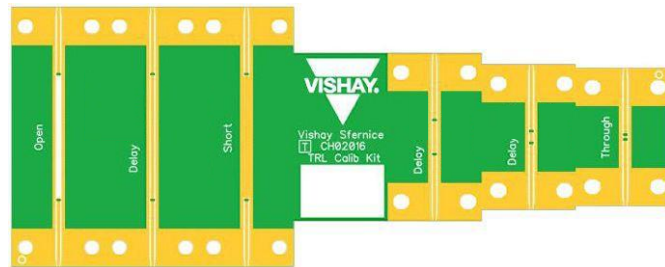
Fig. 6 - Thru reflect line calibration board
